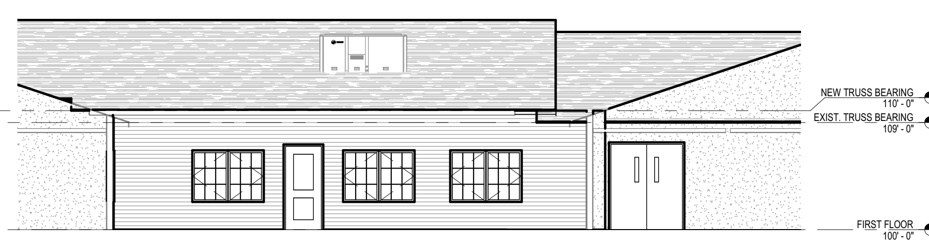
7 UNIT 'C' WEST ELEVATION - SOUTH A4.01 1/8" = 1'-0"
